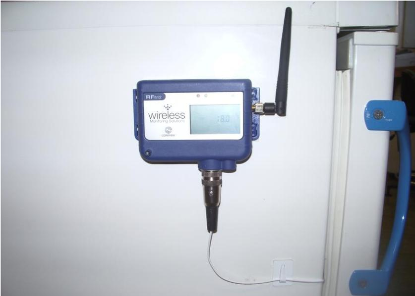
**Note:** Wherever possible use a dedicated port to run the external probe into the equipment (ie Incubator, Freezer, Fridge). If you wish to mount the transmitters on the inside of any equipment please make sure that this is the way that the system was surveyed. It is very important that the position of the transmitters is exactly as it was during the survey to be sure that the system will work.
